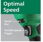
A variable speed trigger and speed dial control allow for easy speed adjustment.
